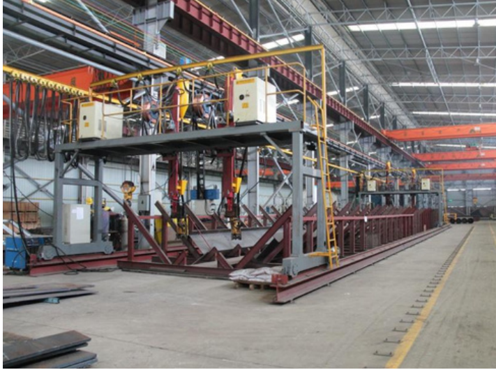
H TYPE STEEL WELDING
