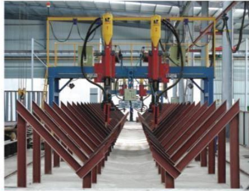
◉ MZG系列MZG-2x1000门型自动埋弧焊机 Mzg Series Mzg-2x1000 Automatic Submerged Arc Welding Machine
