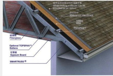
Roofing Type 2 屋面类型2
