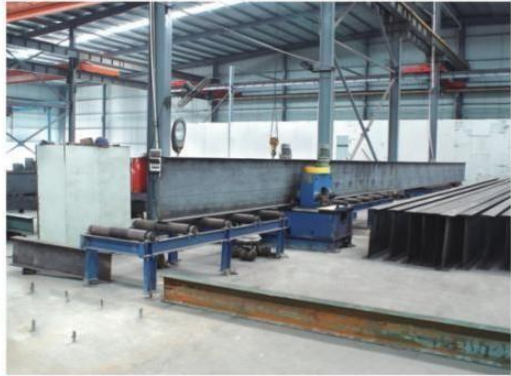
◉ JZ-400A系列H型钢翼缘矫直机 Jz-400a Series H Type Steel Flange Straightening Machine
