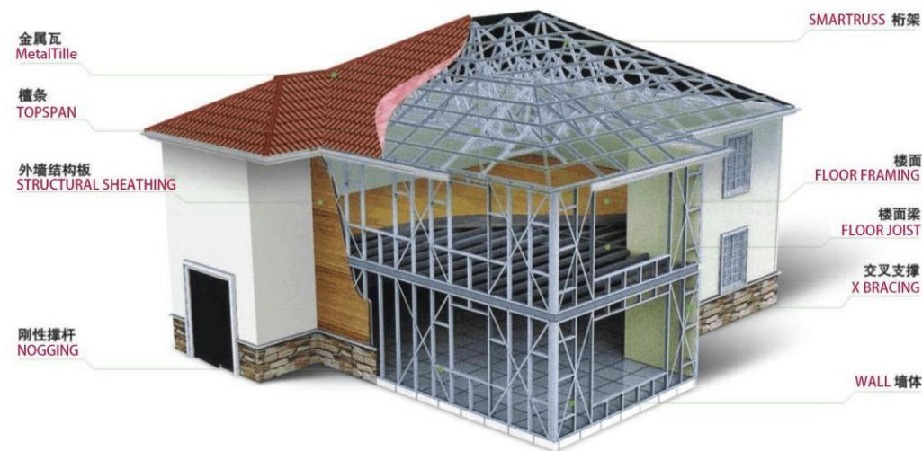
Residential System Components 住宅系统的组成图示
